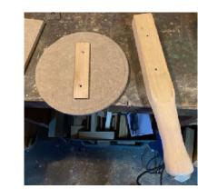
**4** If you want a handle, screw it on from inside, from the thinner backing material into the thicker handle. That means attaching the handle before mounting the glass. Pan head or sheet metal screws avoid having to countersink the thin back support. Locate the screws to avoid impeding the glass. I added a cleat on top but it's not necessary.
