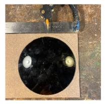
**3** The back support for the glass can be something like 1/4" plywood or particle board, leaving a ¼" extra all around for the adhesive bead to spread. You can leave the support square or trim the corners or cut a circle with power or hand tools according to your resources.
