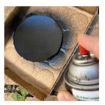
2 Paint the inner concave face black using spray can lacquer or brush on acrylic paint, 2 coats should make it opaque. Clean the surface with Windex or alcohol before you paint: smudges will show because they come in front of the black coating.
