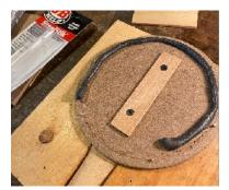
**5** The glass needs to be pressed into a bead of silicone caulk or thick epoxy. Apply pressure gently and gradually to avoid breaking the glass.
